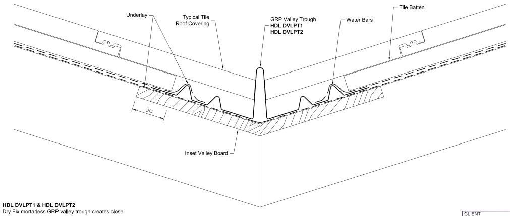
cut appearance on new build and refurbishment. Suitable for all flat and plain tile types. Available in standard lead grey colour.
